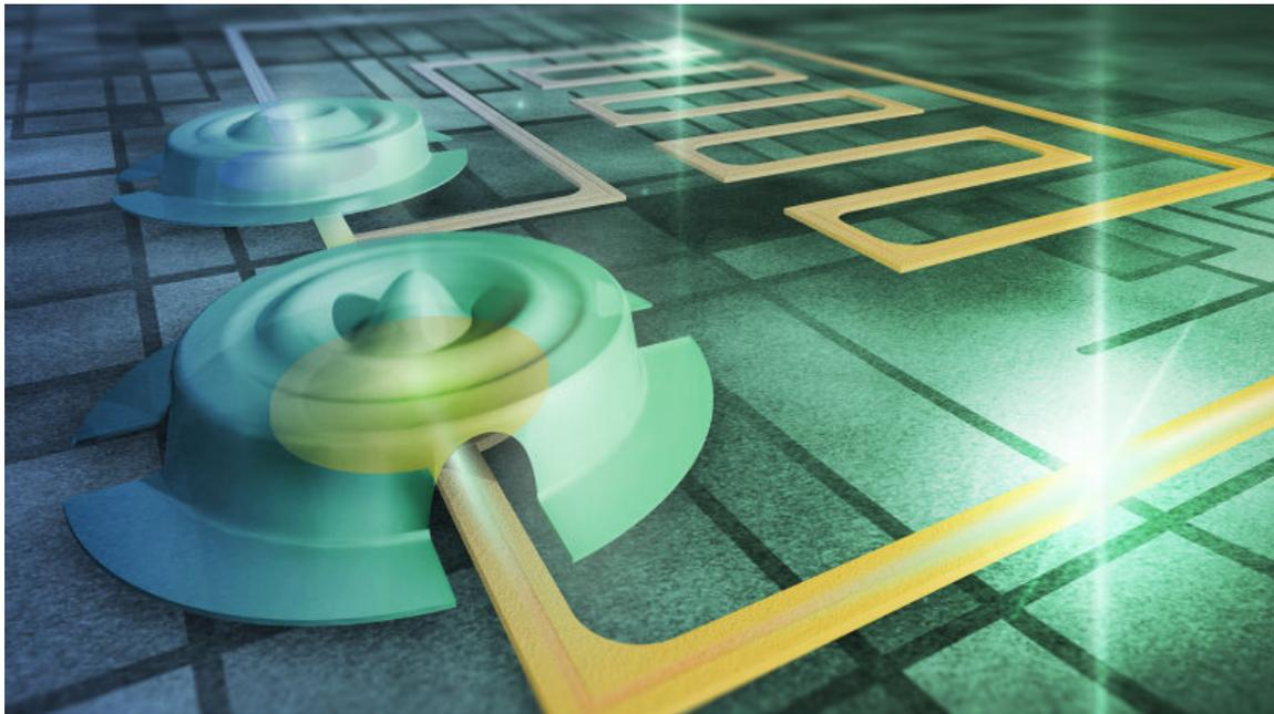
An illustration of one of the experiments, featuring two 15-micrometer vibrating drumheads. Illustration: Aalto University/Petja Hyttinen & Olli Hanhiova, ARKH Architects. (Phys.org)
