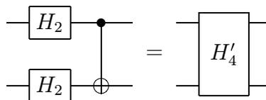
where  $H'_4 = U_{\text{SI}}^{-1} H_4$ . This modified gate is realized by a half-wave plate and a  $\pi$ -mode converter followed by a Mach–Zehnder interferometer with a Dove prism in one arm.
