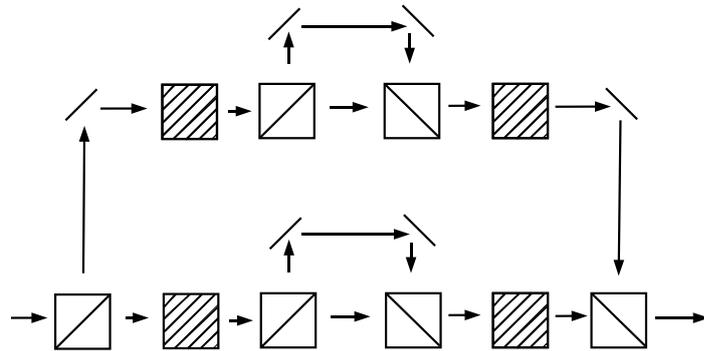
**Figure 4.** Physical implementation of step operator. There are four paths here. The hashed boxes represent SIs and the boxes with diagonal lines represent polarizing beam splitters. The wave plates that transform the photon polarization and OAM have been removed for clarity.
