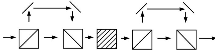
**Figure 3.** Physical implementation of the step operator. There are four paths here. The hashed box represents an SI and the boxes with diagonal lines represent PBS. The wave plates and mode converters that transform the photon polarization/OAM have been removed for clarity.
