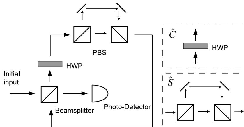
**Figure 1.** On the left-hand side is the experimental setup used by Schreiber *et al* [22]. On the right-hand side are the physical realizations of the coin and step operators. In this work, we will replace the half-wave plate and the Mach–Zehnder interferometer with components that act on an extended Hilbert space. The initial state preparation is not shown.
