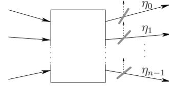
FIG. 2. Schematic illustration of the photon loss model being used. The losses suffered by each output mode are represented by fictitious beam-splitters with transmittivities  $\eta_d$ . The beam-splitters incorporate the combined effect of imperfections of the multiport devices and effects influencing the state during propagation between the multiports (e.g., scattering and absorption).
