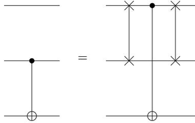
**Fig. 3.** Construction of a CNOT gate between two atomic qubits, using two SWAP gates
