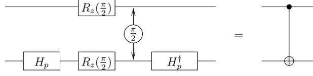
**Fig. 2.** Construction of CNOT gate using a  $J$ -coupling interaction
